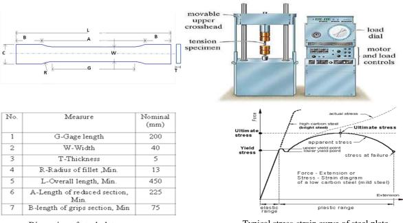
Dimension of steel plate coupons
